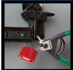
The Unisto Cutter Kit provides everything you need for the fast and safe removal of heavy duty bolt and cable seals.
